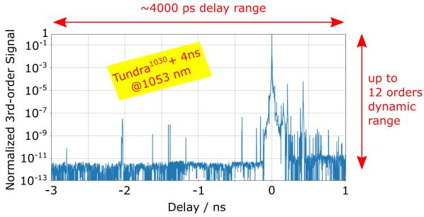
Tundra1030+ 4ns contrast measurement at 1053 nm featuring a 4000 ps delay range, here shifted to negative delays to maximize information about pre-pulses. We characterized the PHELIX 500 TW laser at the Gesellschaft für Schwerionenforschung (GSI) in Darmstadt (Germany) with a pulse duration of 500 fs at 10 Hz repetition rate. The measurement demonstrates the low noise level of our Autocorrelator.
