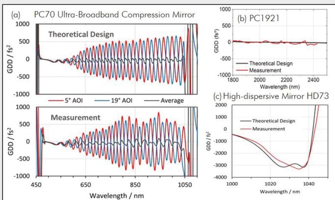
In contrast to other devices GOBI is able to resolve strong GDD oscillations. Note that differences between measured and theoretical curves reflect tolerances in the manufacturing process of the coatings.
